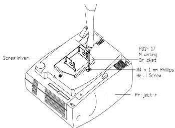
Using a screwdriver, secure the PDS-017 mounting bracket using four (4) M4 x 10mm Phillips Head screws. Do not over tighten these screws. Overtightening the screws may result in damaging the threaded inserts on the projector.
